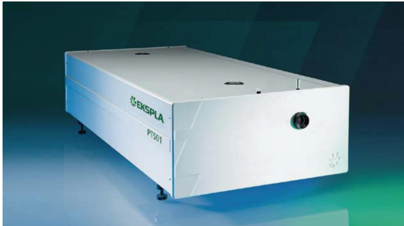
PT501 series laser systems integrate a picosecond optical parametric oscillator (OPO) and a pump laser in a single compact housing. Mounting the components on the same frame provides a robust solution. It makes laser installation shorter, improves long-term stability, and reduces maintenance costs.
