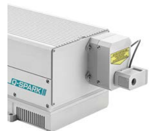
Attenuator and pulse energy monitor attached to the laser head
