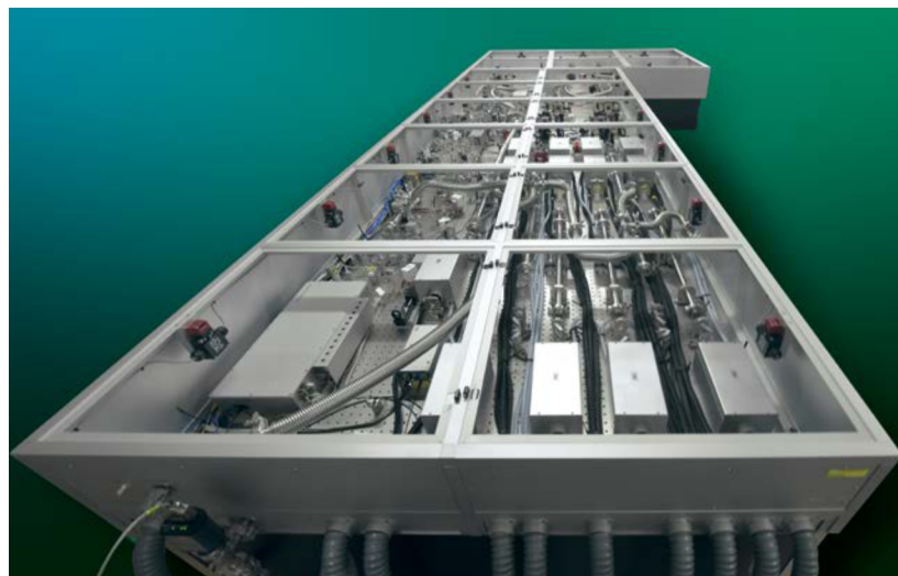
Fig 2. Integrated multi-channel high energy PicoFlux pump lasers into OPCPA
