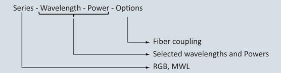
E.g. MWL-(638-20-520-30-473-40): Computer-controlled multi-wavelength laser with 20 mW@ 638 nm, 30 mW @ 520 nm, 40 mW @ 473 nm and FC connector.
