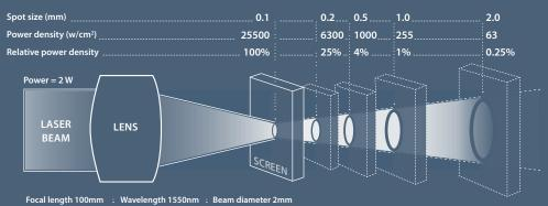
Approximate minimum power density required to observe an infrared laser source from a distance of one meter:
