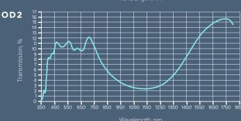
For optional use at higher than about 200 mW lasers (@1064nm) (does vary with wavelength, refer to spectral sensitivity curve), you may consider using following filters to avoid sensor overfilling ("light flooding") issues and still ensure high visibility ofyour surroundings as the filter maintains high transmittance in the visible region compared to regular neutral density filters.
