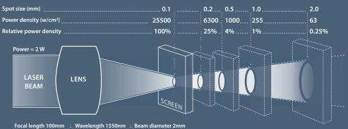
Approximate minimum to observe an infrared laser source from a distance of one meter:
