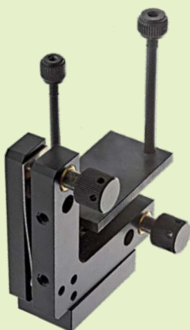
Mount for fine tuning of TK8 crystal ovens angle. The tuning range is \pm 2.5^\circ .
